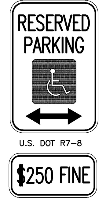
ILLINOIS STANDARD R7-1101 TO BE MOUNTED BELOW R7-B SIGN NOTE: 1.) SIGNS SHALL MEET ALL OF THE REQUIREMENTS OF THE ILLINOIS ADMINISTRATIVE CODE, LATEST ISSUE FOR HANDICAPPED PARKING SIGNS. 2.) FINE IMPOSED MAY BE HIGHER IF REQUIRED BY LOCAL ORDINANCES. A.D.A. PARKING SIGN INSTALLATION NOT TO SCALE
